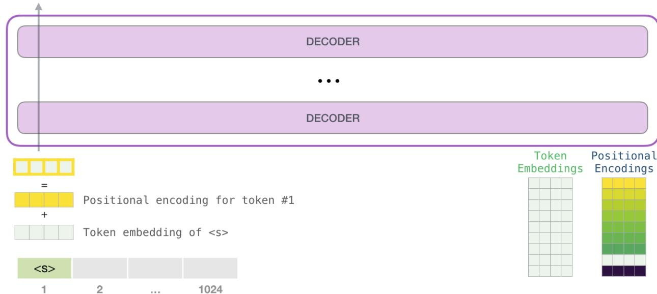
Sending a word to the first transformer block means looking up its embedding and adding up the positional encoding vector for position #1.
